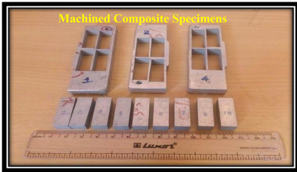
Fig. 3. Machined Al7075 alloy–10-wt.% ZrO 2 composite.
